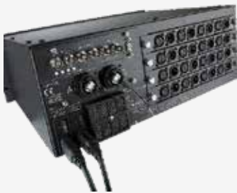
2 x Digico local rack, 32 in, 40 out, 16 AES in/out.
