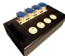
Electrical DB Distribution box 1 x 32A single phase in 4 x 16A and 4 x 13A single phase out.
