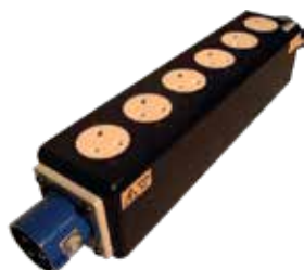
Electrical DB Distribution box 32A single phase in 6 x 13A single phase out.
